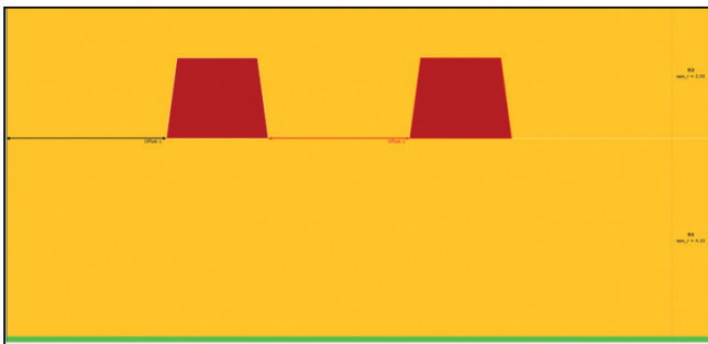
Figure 8: Cross-Section of Differential Pair Tracks Analyzed within Zuken SI Verify. Thickness and cross-section shape are highly significant for closely-coupled differential pairs.
